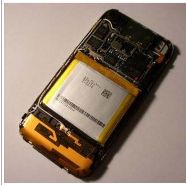
Also remove the metal cover over the comm board. This is all the disassembly you have to do. If you feel like being safe, desolder the battery red lead. I didn't :)
