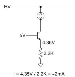
This circuit has a current drift over temperature because of the -2.2mV/Deg-C of the Vbe of the transistor. This can be minimized (As a percentage) by making the voltage across the setting resistor as large as possible. As shown, the typical swing would be:
