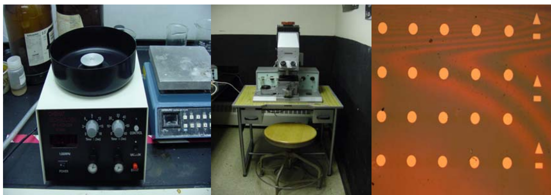
Figure 28: Spin coater, hot plate, mask aligner, and dot pattern after soaked in developer.
