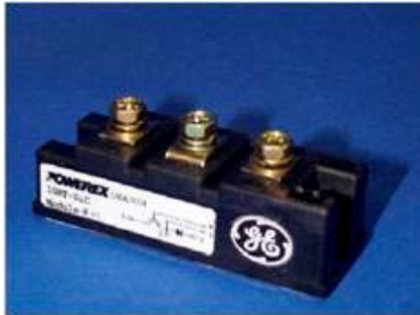
GE/Powerex Si IGBT/SiC Diodes: Si Powerex PT IGBT: 600V/1200V, 75A Single Chip SiC GE Diode: 600V, 20A, 6 Dies in || Each Die is a 5 \mu m Epi, Medium Size 800 \mu m x 800 \mu m
