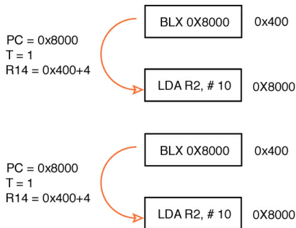
Fig. 10 Branch Exchange and Branch Link Exchange Instruction Operation
