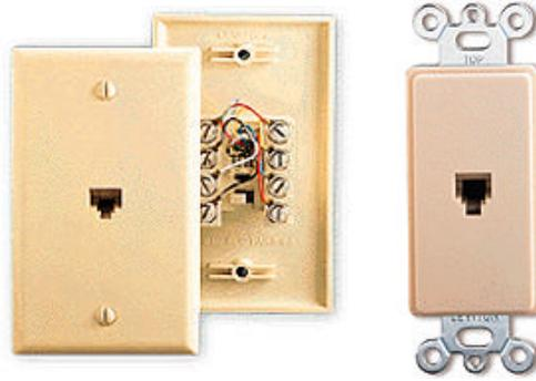
The **flush jack** is flat, like an electrical outlet, and is usually installed in new construction, with wire concealed inside the wall. Flush jacks are available in a variety of colors, for two, three or four pairs of wire, and in both standard and "Decora" styles (at right, above).
