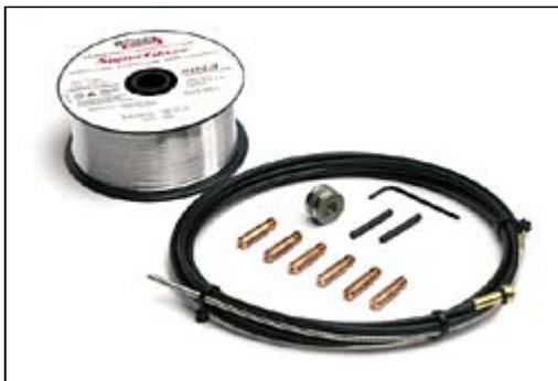
Do not use other diameter wires. Specifically, you should avoid 0.030" wire (it is difficult to feed) and 3/64" wire (these compact machines do not typically produce enough current to reliably melt this diameter of wire).
