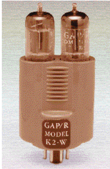
The first commercial op amp. Photo courtesy of Dan Sheingold and Analog Devices Inc.
